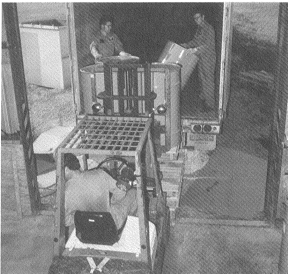
One program successfully completed during 1988 was the repackaging of lithium hydroxide. Plant crews safely repacked several hundred thousand cardboard drums of the compound into steel drums for improved permanent storage. The drums were then relocated to upgraded warehouses.
